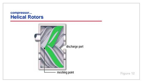
Viewing the compressor from the top shows that rotation of the meshed rotor lobes drives the trapped refrigerant vapor (to the right) ahead of the meshing point.
